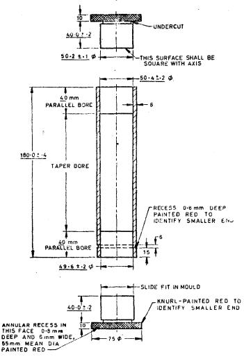
NOTE 1 — All surfaces should be smooth and free from tool marks. NOTE 2 — Material — mild steel.
