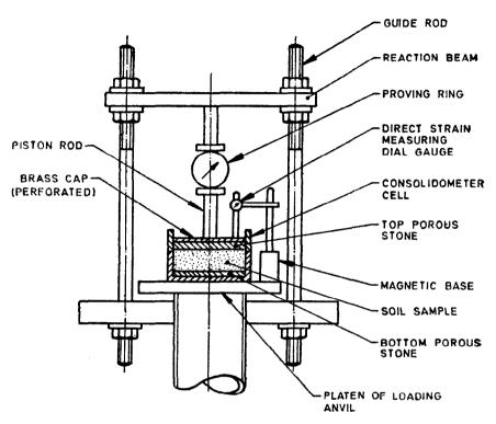
Note — The above is only an illustrative set up. Any suitable apparatus which minimises volume changes may be preferred.
